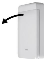
1. Gently pull the button off by hand at the upper end. Then unhook it at the lower end.
